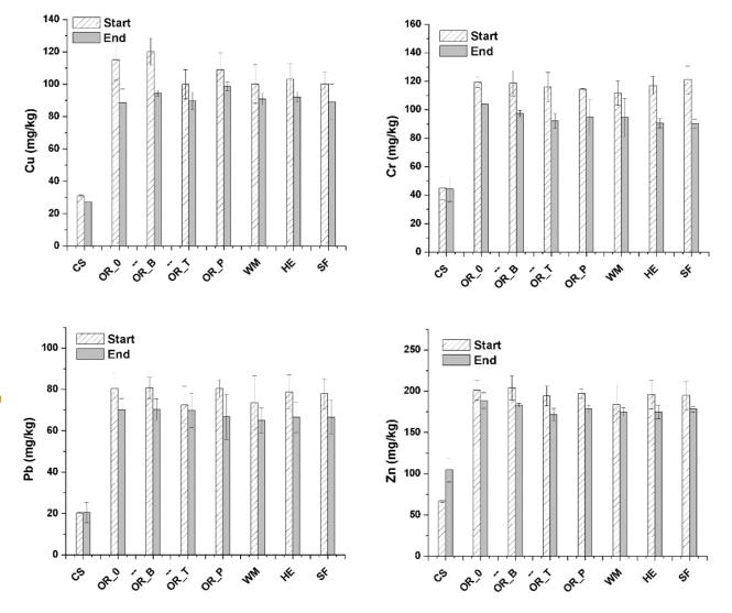
Figure 6 Concentration of Cu, Cr, Pb, Zn (the metals detected in the highest concentrations) at the beginning and at the end of the pot tests for the different investigated conditions (CS: contaminated soil, OR\_0: rapeseed and no PGPR treatment, OR\_B: rapeseed and treatment with Bio Eho PGPR; OR\_T: rapeseed and treatment with Trifender Pro PGPR, OR\_P: rapeseed and treatment with Panorama Bio Plus PGPR, WM: White Mustard; HE: Hemp; SF:Sunflower). Credit: IFVCNS
