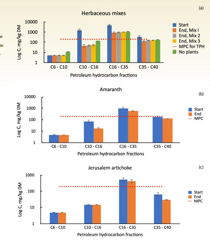
Figure 5 TPH concentrations in the contaminated soil at the start and at the end of the pot experiments performed at BVA facilities, with a) Herbaceous mixes b) Amaranth, and c) Jerusalem artichoke (n=3). Note the logarithmic scale. MPC= Maximum permissible concentration value, according to Lithuanian legislative document LAND 9-2009 (200 mg/kg). Credit: BVA
